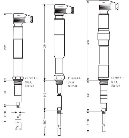
Fig. 1 NRG 16-51, NRG 17-51 with four-pole connector and measuring surface extension
