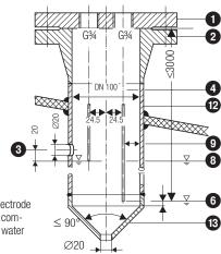
Fig. 11 Protection tube (provided on site) if electrode is used as internal water level-limiter combined with water level control or high water level alarm
