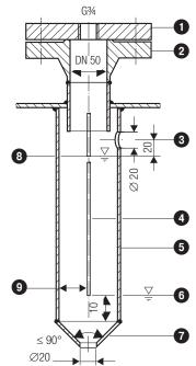
**Fig. 7** Protection tube (provided on site) if electrode is used as internal water-level limiter
