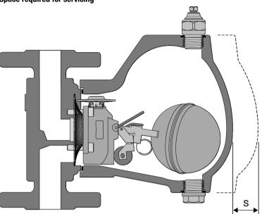
To remove the cover a withdrawal space S of 240 mm is required.
