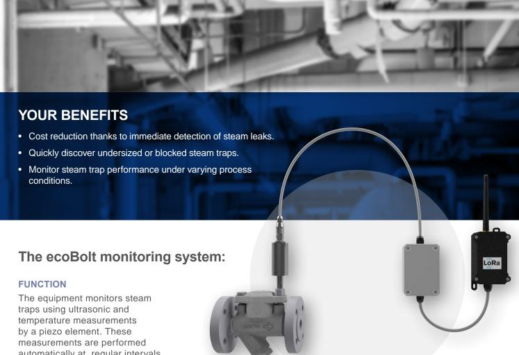
traps using ultrasonic and temperature measurements by a piezo element. These measurements are performed automatically at regular intervals. The measured data is analysed in the LoRa node and transferred to the LoRa gateway (accessory). The data is transferred by LoRa wireless technology via network protocol. The measurement results are analysed on the basis of the sound and temperature values and parameters of the steam trap under test.
