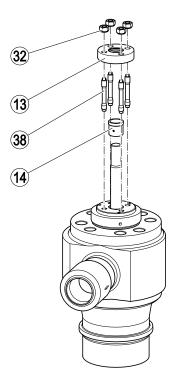
After mounting the stuffing box flange you can fasten the bolts of the stuffing box for the pressure balance with the indicated torque.
