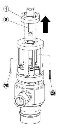
Unscrew the spindle out of the bearing if necessary.
