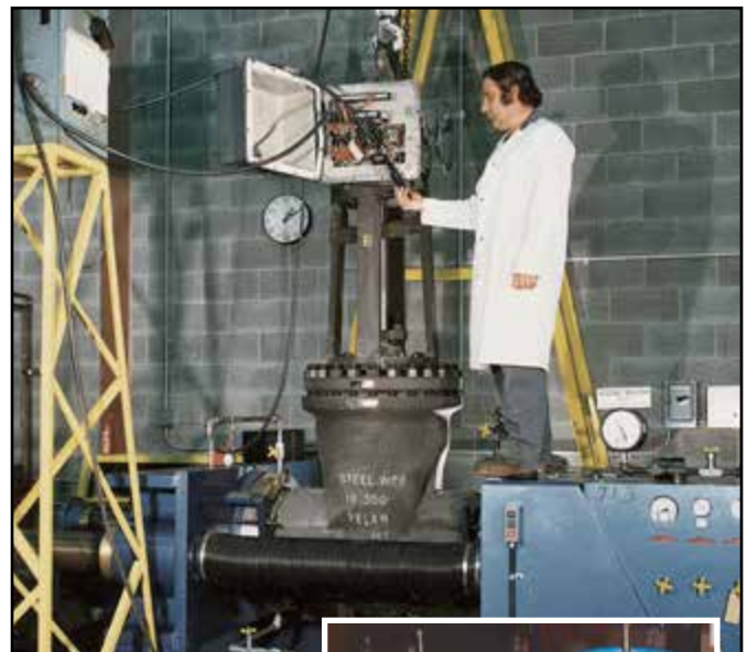
Above: Operational test for electric actuators.
