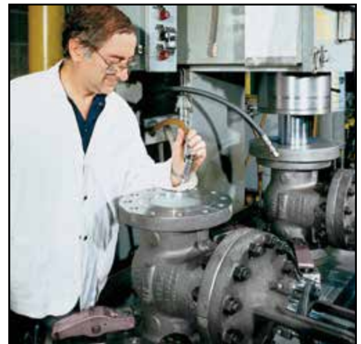
8 After assembly, pressure testing of shell, seats, packing, and backseat to API 598.
