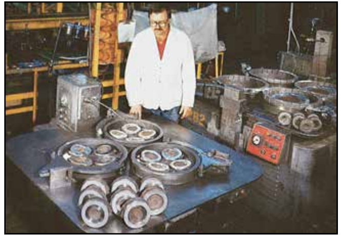
6 Lapping of wedge seating surfaces.
