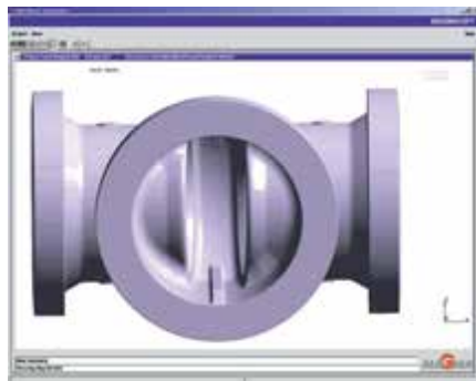
3-D solid model of casting imported into MAGMASOFT® simulation program.
