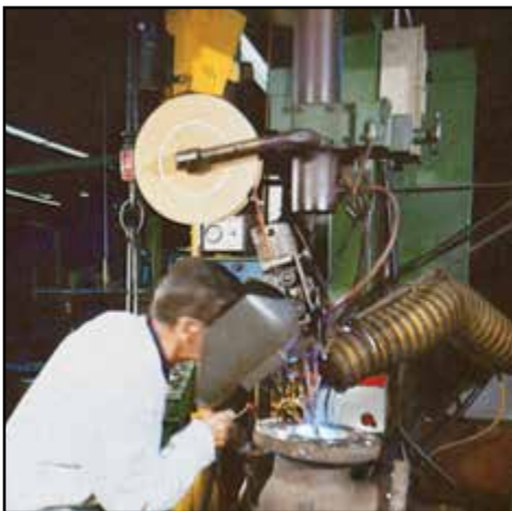
1 Automatic seal welding of CoCr alloy hardfaced seats.
