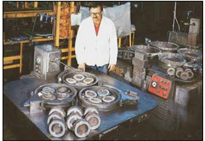
6 Lapping of wedge seating surfaces.
