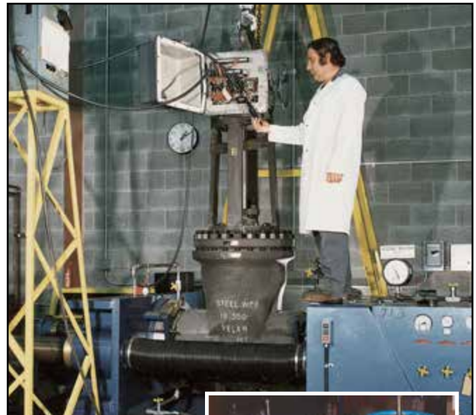
Above: Operational test for electric actuators.
