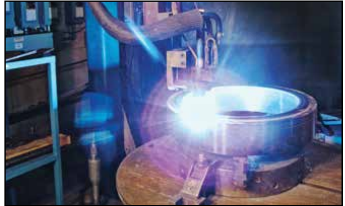
Automatic plasma arc hardfacing equipment for seats.
