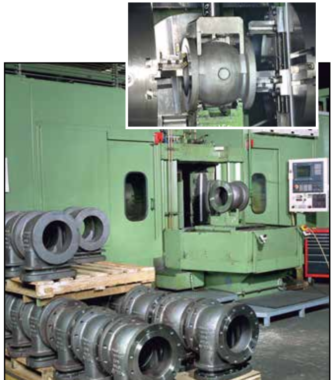
Automatic three-way facing machine.
