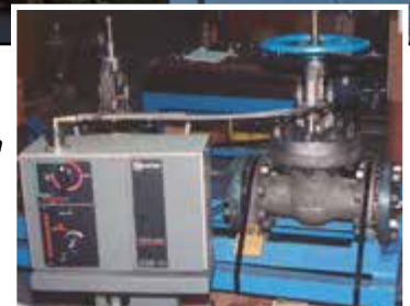
Above: Operational test for electric actuators.
