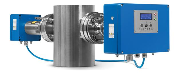
GasEye SO2/CO/H2O is a high performance *in-situ* combined sulfur dioxide/carbon monoxide with parallel measurement of water vapor content analyzer. Suitable for safety applications and process control. 24/7 continuous operation. One flange pair. No sample preparation. No zero drift. No field calibration. Low cost of ownership.
