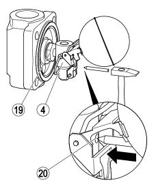
Attach the control unit to the body as described from page 17 onwards.
