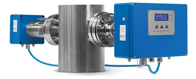
GasEye Cross Duct O2 SC is a high performance *in-situ* oxygen analyzer with separated central unit (SC). Suitable for safety applications and process control. 24/7 continuous operation. One flange pair. No sample preparation. No zero drift. No field calibration. Low cost of ownership.
