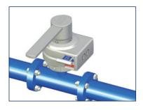
The valve is closed. The lower key **A** (red) can be removed. Upon removal of the key the valve is locked again and can no longer be operated. The upper key **B** (blue) remains trapped in the slot. The state of the valve (closed) is clearly visible from the vacant lower key slot.
