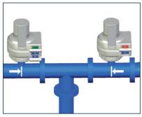
An authorised person inserts the key **A** (red) into the right interlock. The lock is released and the operator can close the right valve. As soon as the valve is closed, the key **B** (blue) can be removed. Upon removal of the key the valve is locked again and cannot be operated. The media in the right pipe can no longer flow on.
