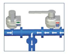
This example shows the switch over from one media (right pipe) to another (left pipe). Any mixing of both media must be avoided.
