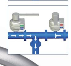
Now the operator inserts the key **B** (blue) into the left interlock. The lock is released and the operator can open the left valve. As soon as the valve is open, the key C (green) can be removed. Now the media can flow in the left pipe. By removing the key, this valve is also locked and can no longer be operated.
