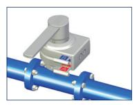
The authorised person closes the valve. During operation, keys  $\bf A$  (red) and  $\bf B$  (blue) are both trapped. As soon as the valve lever is in its final position, key  $\bf A$  (red) is released.
