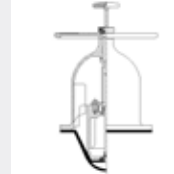
Non-rising handwheel with indicator DN200 - DN300 8" - 12"
