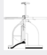
Non-rising handwheel with indicator DN200 - DN350 8" - 14"
