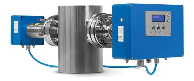
GasEye SO2/HCI is a high performance *in-situ* combined sulfur dioxide and hydrogen chloride analyzer. Suitable for emission monitoring and process control. 24/7 continuous operation. One flange pair. No sample preparation. No zero drift. No field calibration. Low cost of ownership.
