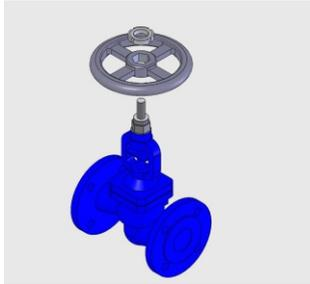
*Remove hand wheel nut and hand wheel*
