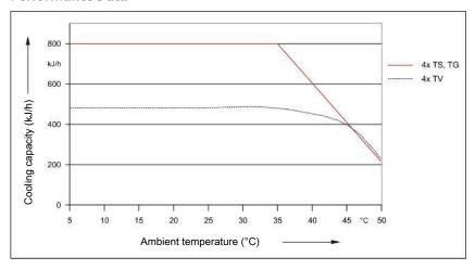
Note: The limit curves for the heat exchangers exchanger apply to a dew point of 65 °C.
