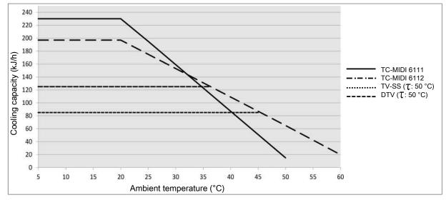
Note: The limit curves for the heat exchangers exchanger apply to a dew point of 50 °C.
