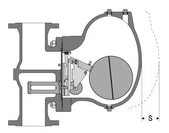
To remove the cover a withdrawal space S of 350 mm is required.
