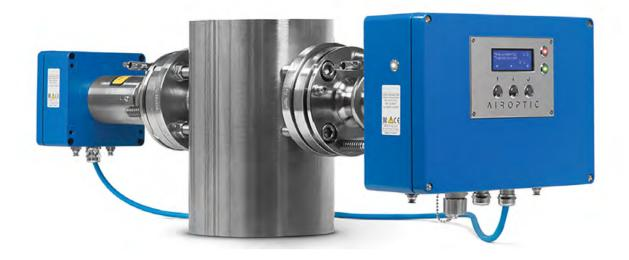
GasEye CO is a high performance *in-situ* carbon monoxide analyzer. Suitable for safety applications and process control. 24/7 continuous operation. No sample preparation. No zero drift. No field calibration. Low cost of ownership.
