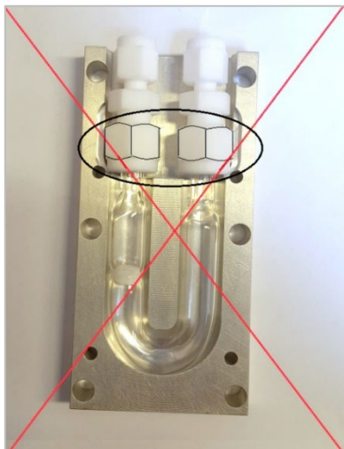
Figure 12. Incorrectly aligned connector nuts
