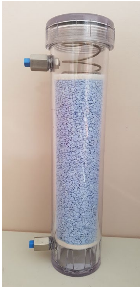
Figure 36. Absorption dryer material
