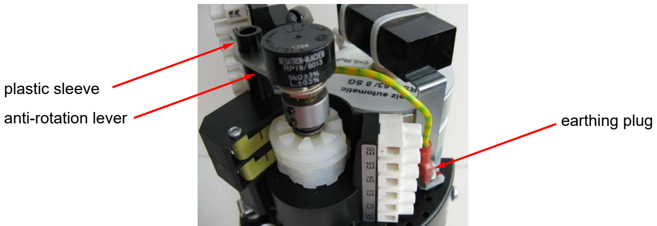
Fig. 17: Fitting a potentiometer to the 2EZ assembly
