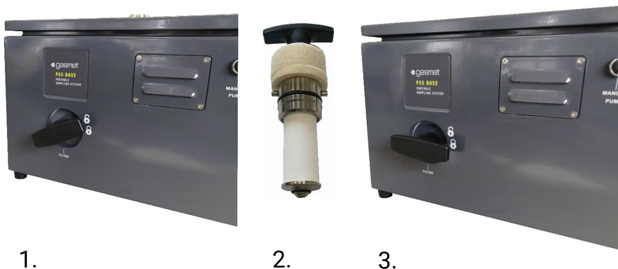
Figure 5. Changing the sample filter. 1. Filter housing handle in open position. 2. Sample filter and filter housing. 3. Filter housing handle in closed position.
