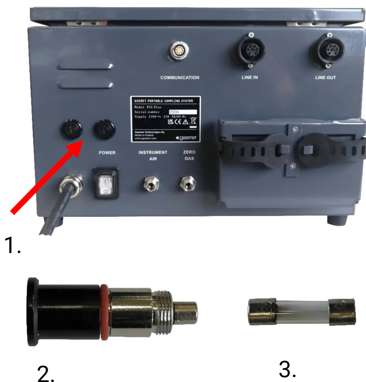
Figure 6. Changing the fuses. 1. Location of fuses. 2. Fuse holder. 3. Fuse.
