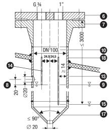
Fig. 6 Protection tube (provided on site) for installation inside the boiler and in combination with other GESTRA equipment
