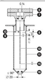
**Fig. 4** Protection tube (provided on site) for installation inside the boiler
